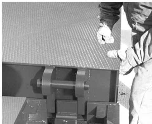
Figure 3-6. Pin and Receptacle Interface
