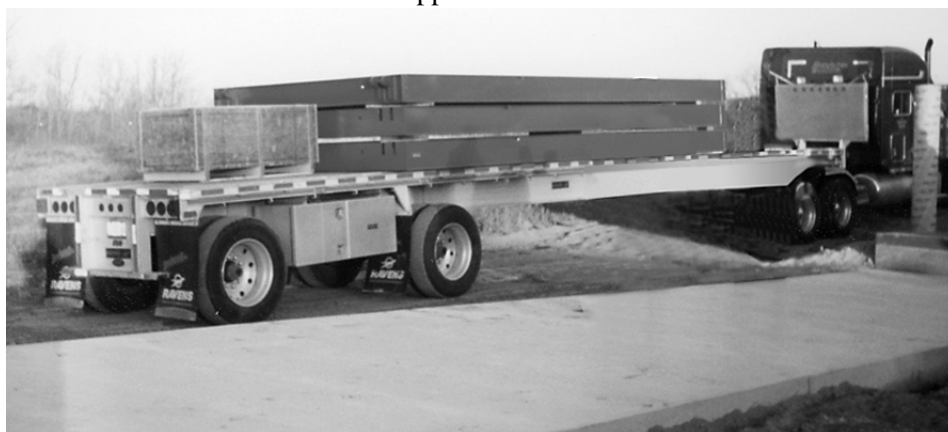
Figure 3-2. Weigh Modules Ready for Removal and Installation
